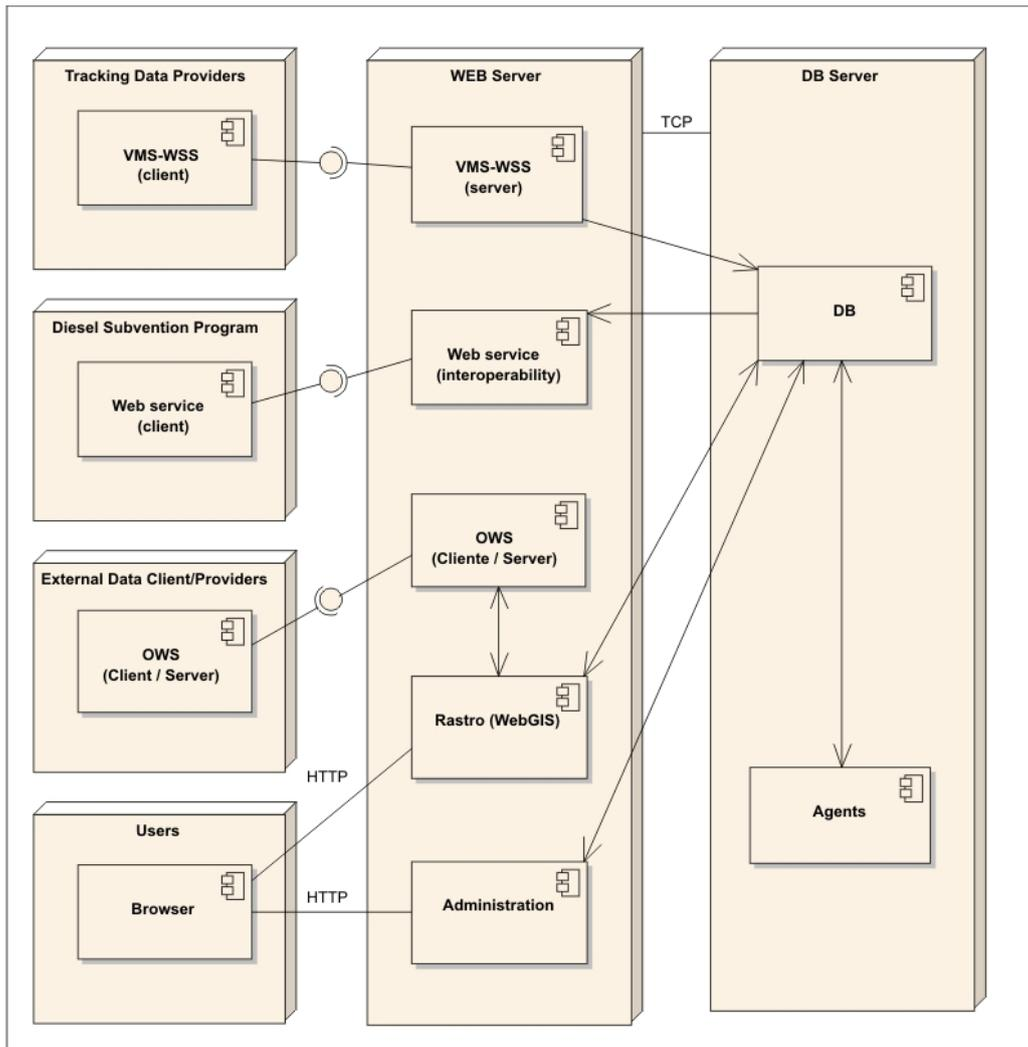
Figure 4: System's architecture.
