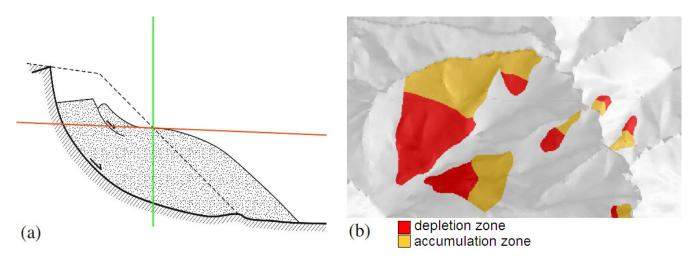
Figure 1. Division of a landslide in accumulation and depletion zones: (a) sketch of a ground profile, where the red line represents the ideal tangent line in the flex point of the slipped surface; (b) results of the proposed procedure.
